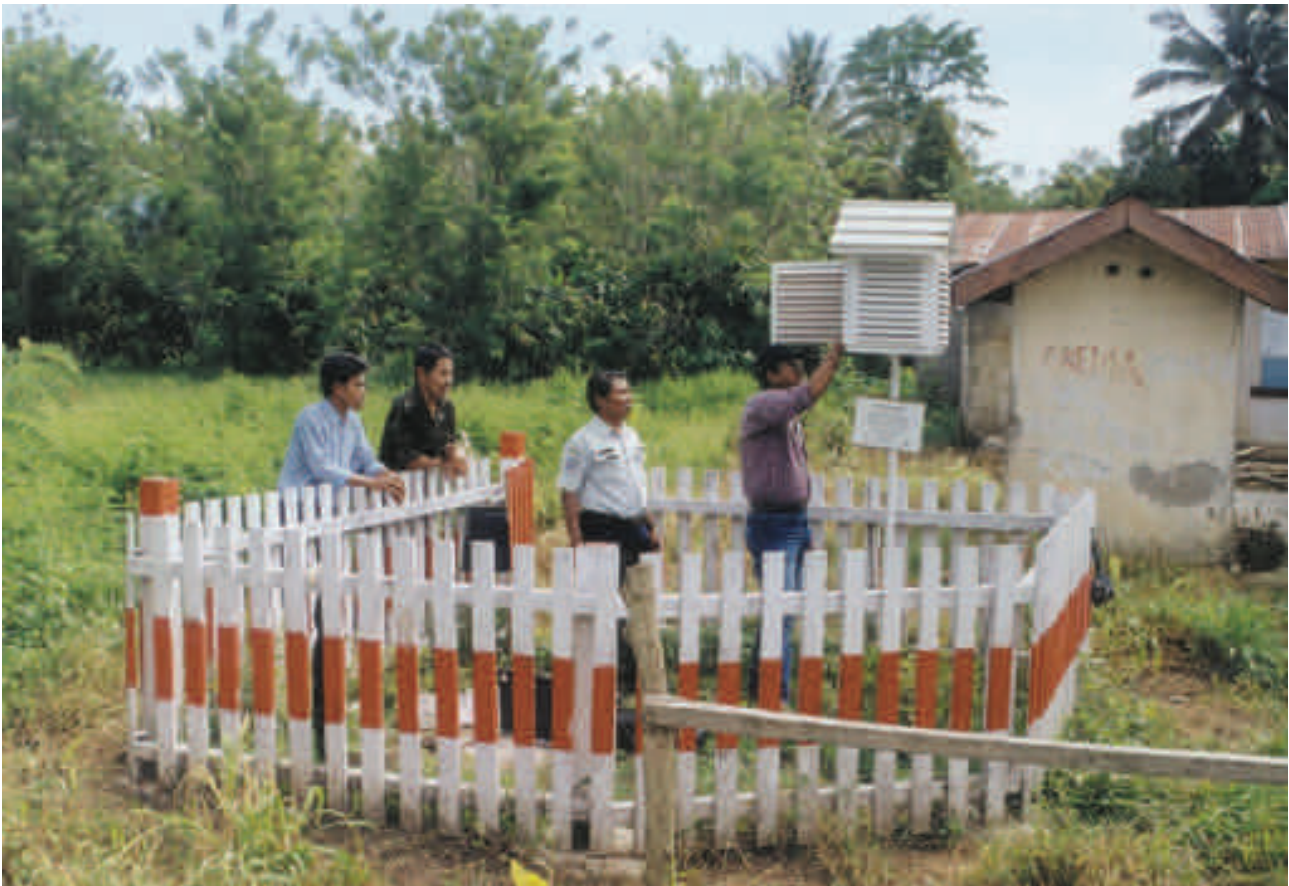
Photo 1. Data readout at one of eight IMPENSO climate stations in co-operation with the Indonesian meteorological service. The establishment and maintenance of the stations involve the local population.
